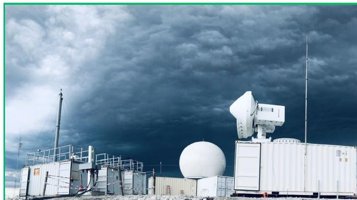
The main TRACER observatory will be the first ARM Mobile Facility, seen here during a 2018–2019 field campaign exploring the life cycles of large convective storms in north-central Argentina.
