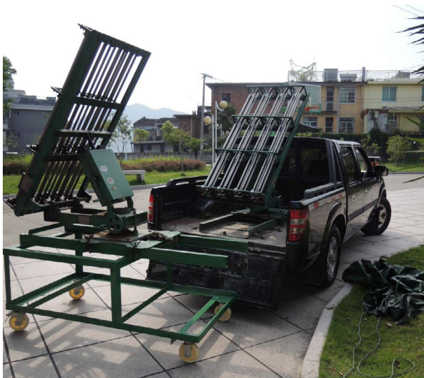
Fig. 2. Mobile rocket launchers used for precipitation enhancement. Source: taken by the author.
